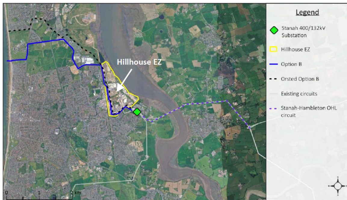
Figure 1-2: Option B Rossall Landing with Hillhouse/Stanah Onshore Cable Route and Surrounding Network
