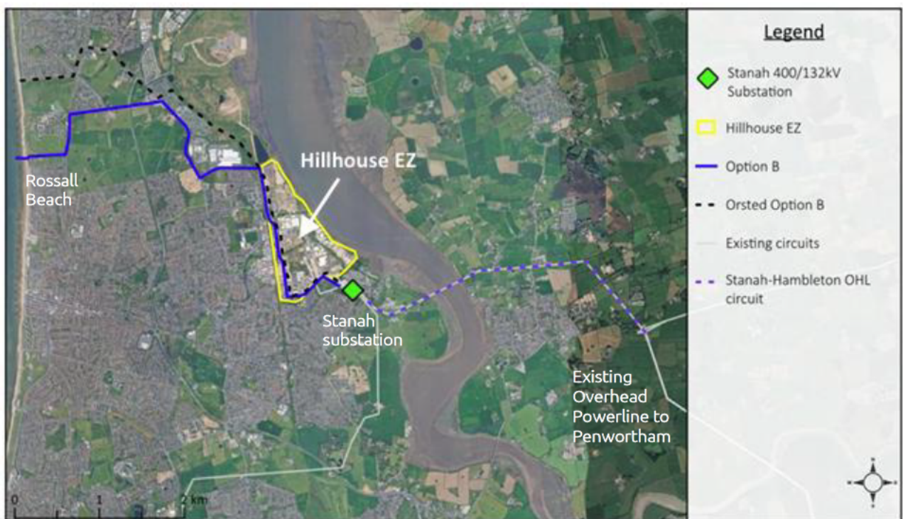
Figure 3.2: Option B Rossall Landing with Hillhouse/Stanah Onshore Cable Route and Surrounding Network
